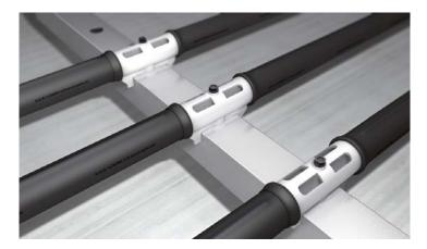
**MAGNUM®** diffusers can be installed on rectangular or round headers with 30 mm or 38 mm (1.18" or 1.50") outlet openings. We offer connectors for DN 80, 100 and 125 mm (3.15", 3.94" and 4.92") diameter round headers and 80, 100 and 120 mm (3.15", 3.94"and 4.72") rectangular headers.
